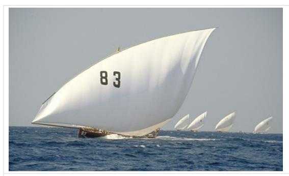
What a sight! The racing dhow *Sirdal* outpaces four running mates as they all head for the finish line. The *Sirdal*'s mainsail is almost perfectly trimmed, with barely a ripple. Look closely at the topmost planking on the side facing the wind (the windward gunwale). It is just barely above the water line.
